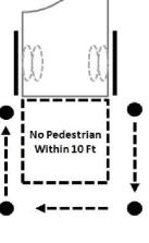
Walk to other side of truck keeping 10' of distance behind back of doors. Never get directly behind back of truck with doors open.
