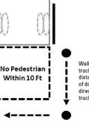
Walk to other side of truck keeping 10' of distance behind back of doors. Never get directly behind back of truck with doors open.
