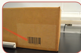
High-speed laser imaging onto water-based Reveel™ coating.
