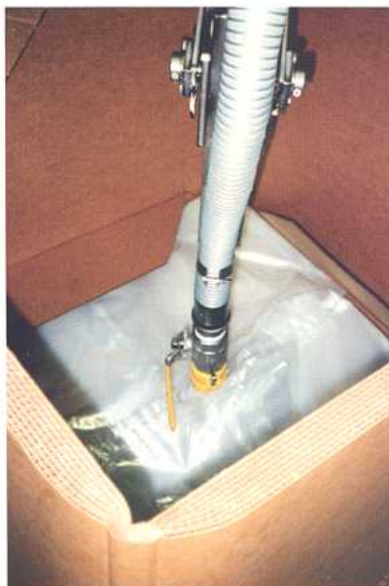
Fish oil takes only about 15 min tops to fill into the 260-gal IBC using a special articulating arm filling system.
