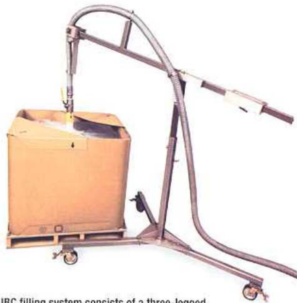
IBC filling system consists of a three-legged mast and boom to support a hose from the fish-oil holding silo to the IBC's filling valve.
