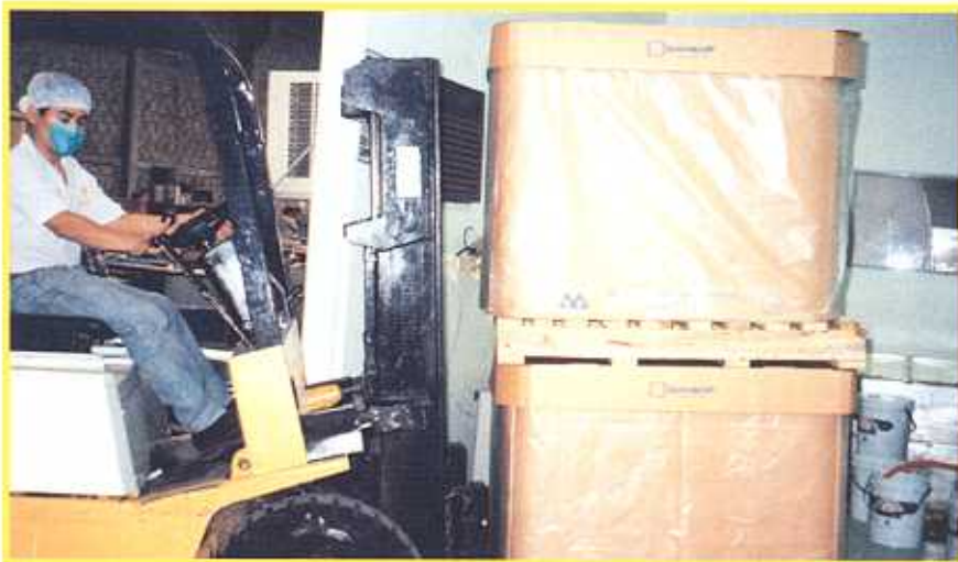
Filled, shrouded and capped IBCs containing honey are stacked two-high in Hansa's warehouse. Withstanding 30 tons of compression, the IBC can be stacked up to four-high.
