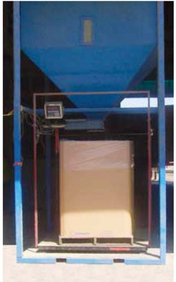
Blending assorted grass seed varieties that are weighed and fed into the bag-lined 1,000-lb totes for storage and mixing, Doerfler Farms reduced labor and handling over using 50-lb bags alone. Each collapsible tote can be reused over and over.
