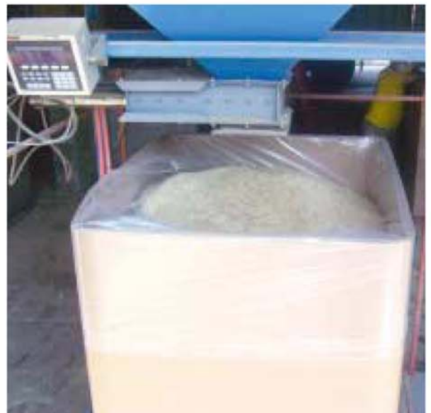
Blending assorted grass seed varieties that are weighed and fed into the bag-lined 1,000-lb totes for storage and mixing, Doerfler Farms reduced labor and handling over using 50-lb bags alone. Each collapsible tote can be reused over and over.
