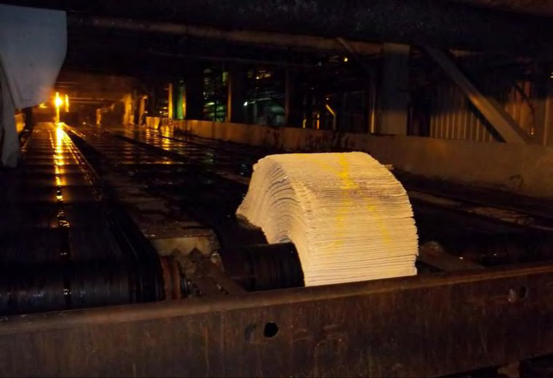
Bales are loaded onto the conveyor belt to be processed
